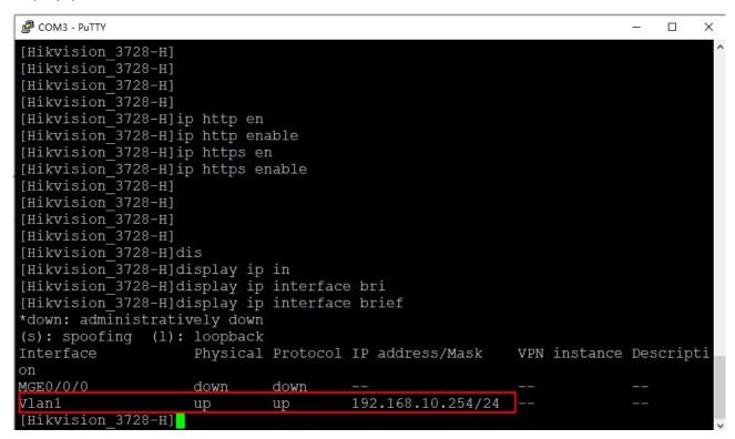
The VLAN 1 is the management VLAN by default, input these commands to change the IP Address.
